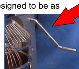
Picture 3. The handle and bowl of the machine must be raised to engage the electrics of the mixer.
